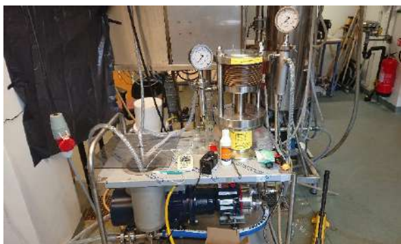
FIGURE 12. The Alfa Laval test unit used for microfiltration.
