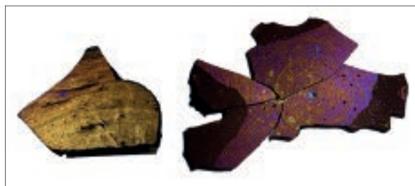
FIGURE 4. A combination of thin film hydrochars (golden and blue) attached to the spherical hydrochars (black) prepared by hydrothermal carbonization of glucose and iron(II)sulfate.
