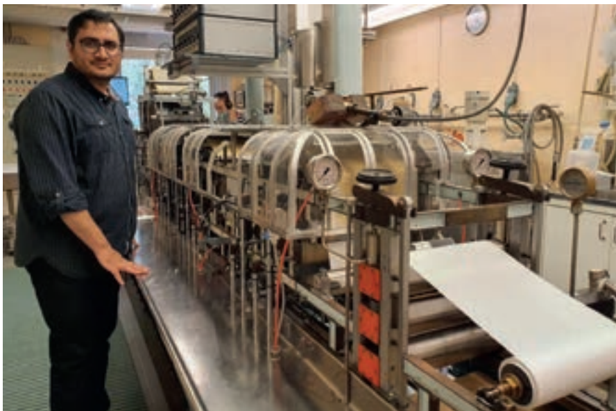
FIGURE 6. Pilot scale production cellulose-metal organic framework filters on XPM at RISE MoRe Research.
