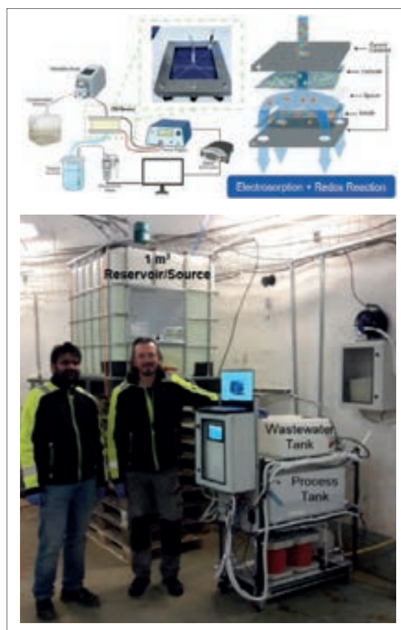
FIGURE 9. CDI-modules used in the tests: left – lab scale device; right – pilot-scale plant with two CORE® CDI modules.
